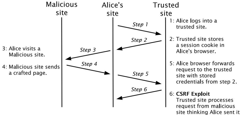
Figure 1: Steps in a cross-site request forgery attack
